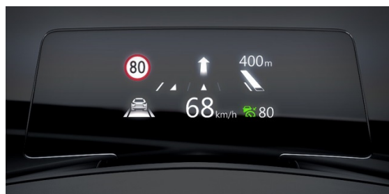
Fig. 8 Traffic Sign Recognition System
