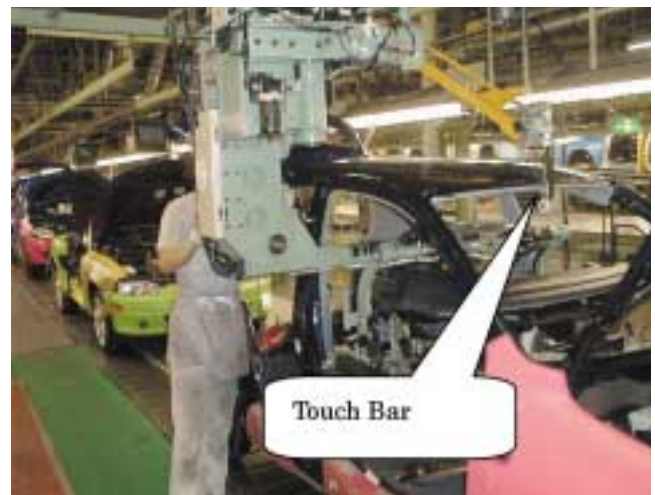
Fig.4 Conveyor Following at IPM Install
