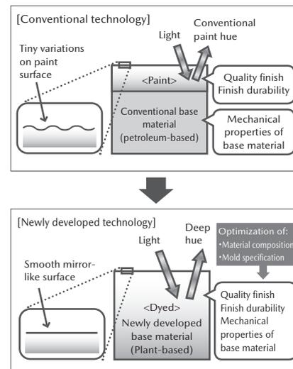
q 2018: New technology for two-layer molding of pattern designed bio-based engineering plastic
