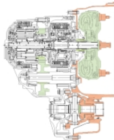
Fig.10 Sectional View of 6EAT
