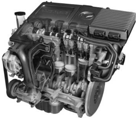
Fig.2 MZR 1.3L Miller Cycle Engine
