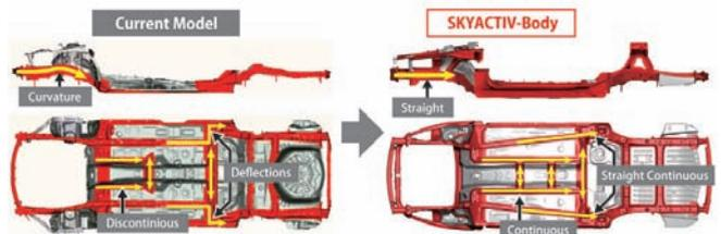
Fig.3 Straightening of Basic Framework and Continuous Framework Structure
