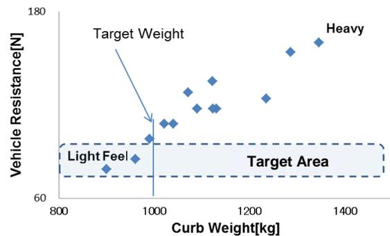
Fig. 6 Curb Weight and Vehicle Resistance
