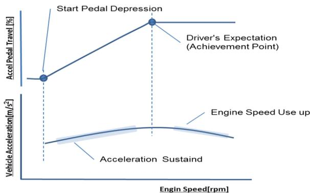
Fig. 2 Acceleration and High Engine Speed Use up
