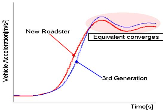
Fig. 9 Vehicle Acceleration of Previous and New Roadster
