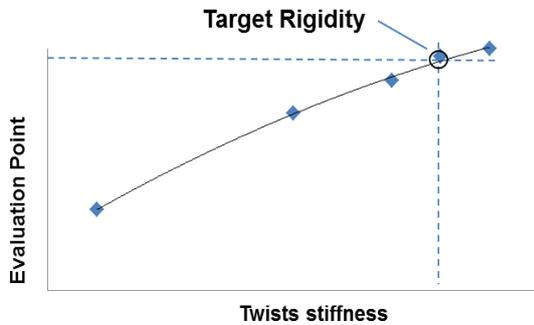
Fig. 8 Torsion Rigidity of Driveshaft Contribution Rate
