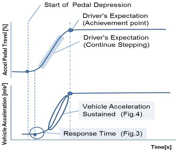
Fig. 1 Basic Concept of Driver's Expectation and Reaction
