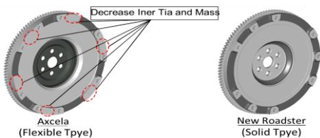
Fig. 10 Flywheel Comparison between Axcela and New Roadster
