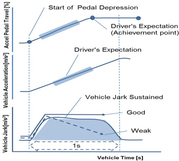
Fig. 4 Development Target of Vehicle Jerk Duration
