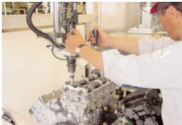
Fig.5 Nutrunner for High Torque Use
