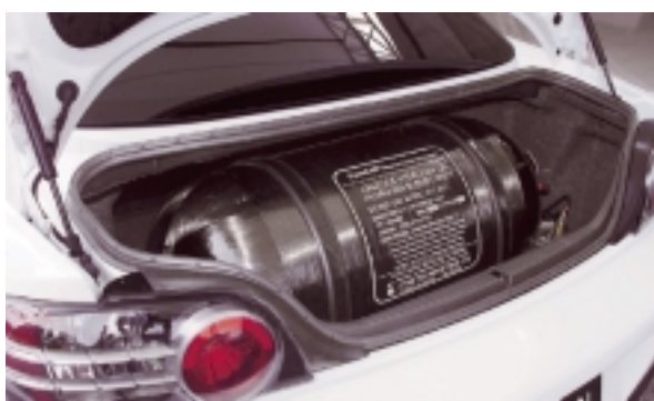
Fig.10 High-pressure Hydrogen Tank
