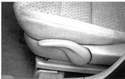
Fig.6 Pump type operation for seat lifter
