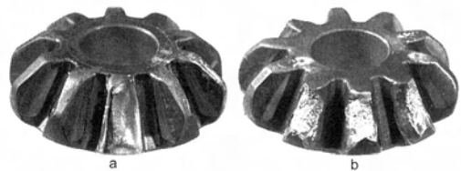
Fig.1 Impact Fatigue Failure (a) and Spalling Failure (b)
