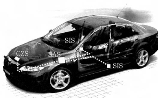
Fig.8 Location of Airbag Sensor
