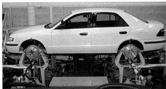
Fig.2 16 Channel Multi-Axis Road Simulator
