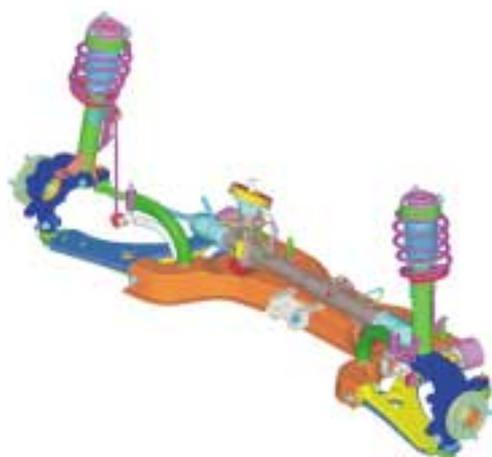
Fig.1 Front Suspension & Steering
