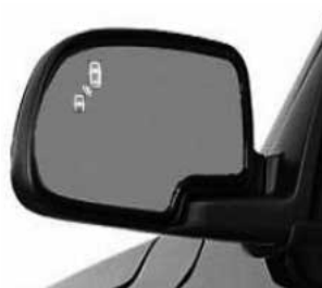
Fig.6 Display Position of Blind Spot Monitoring
