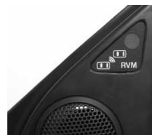
Fig.7 Display Position of Rear Vehicle Monitoring
