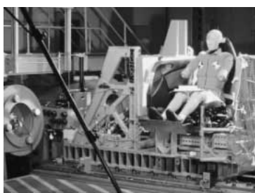
Fig.1 Side Impact Crash Simulator
