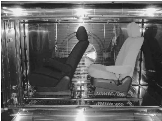
Fig.5 Test Equipments (2m 3 Chamber)
