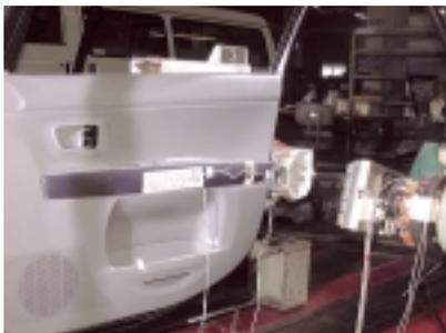
Fig.8 Door Impact Test
