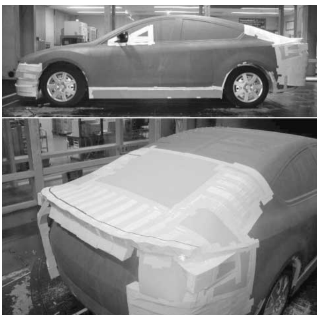
Fig.6 1/1 Scale Model with Aerodynamic Improved Parts
