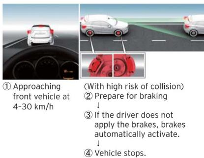
Fig.8 Smart City Brake Support
