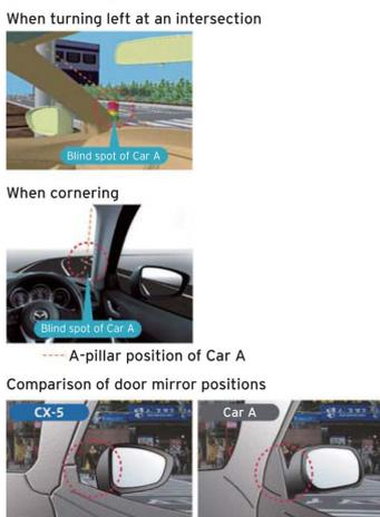
Fig.7 Front View Improvement by A-pillar Form
