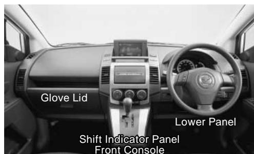
Fig.10 Bioplastic Parts
