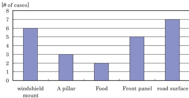
Fig.4 Vehicle Areas Causing Damage in Pedestrian Fatal Accidents<sup>(3)</sup> (Over AIS 3)
