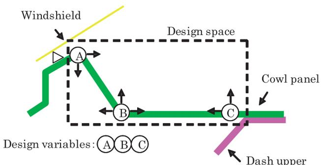
Fig.11 Design Space & Design Variables for Cowl Panel
