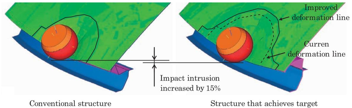
Fig.17 Comparison of Windshield Deformation
