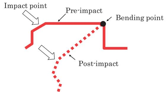
Fig.15 Deformation of Cowl Panel that Achieves Target
