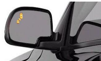
Fig.3 Indication of Car in Blindspot Area or Approaching to it
