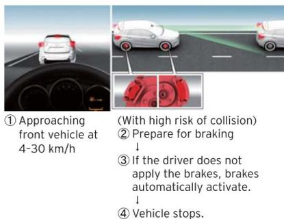
Fig.8 Smart City Brake Support
