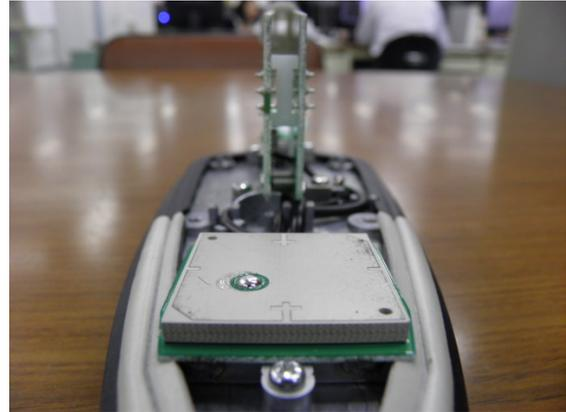
Fig.8 Patch Antenna for Sirius Radio Reception
