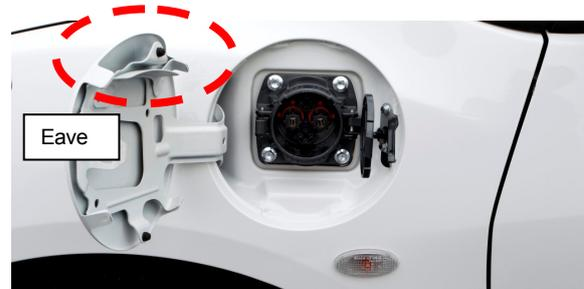
Fig.10 DC Charge Inlet (Front Fender LH)
