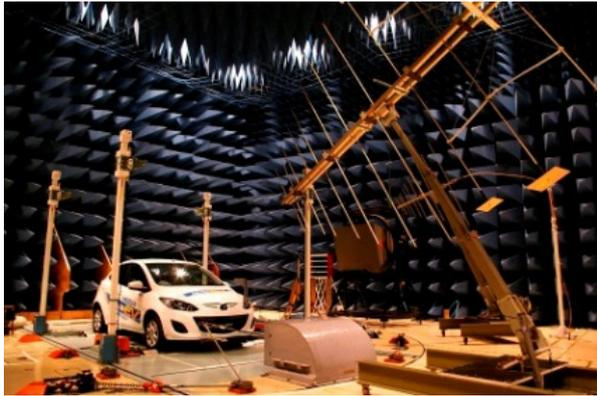
Fig.15 EMC Test
