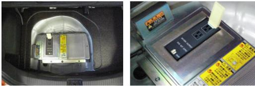
Fig.12 100V Electric Supply System
