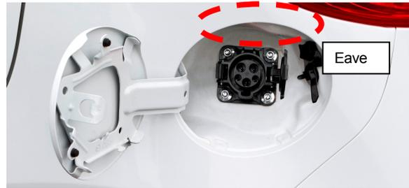
Fig.9 AC Charge Inlet (Rear Fender LH)
