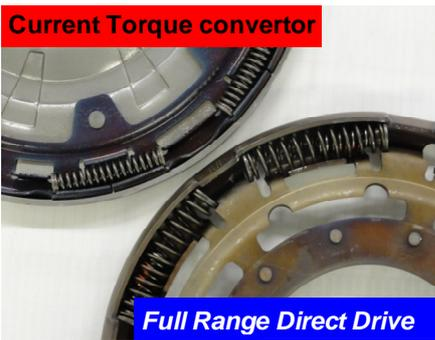
Fig.4 Comparison with Full Range Direct Drive Damper
