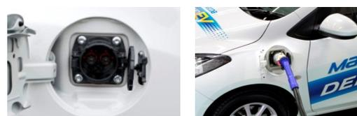
Fig.11 High Speed Charge Lid
