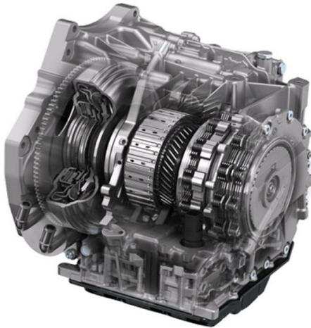
Fig.1 Phantom View of SKYACTIV-DRIVE
