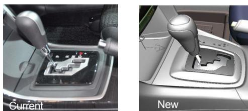
Fig.4 AT Shift Lever Layout
