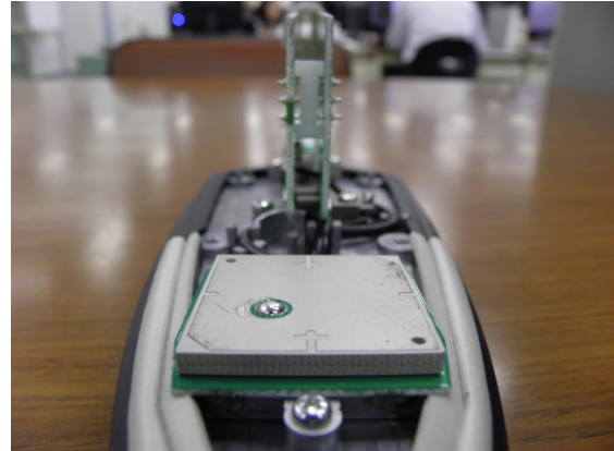
Fig.8 Patch Antenna for Sirius Radio Reception
