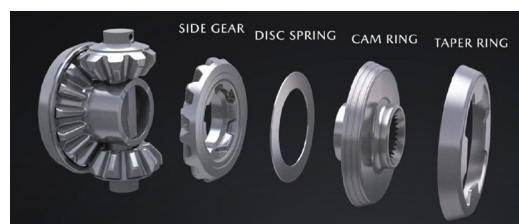
Fig. 2 Components of Asymmetric LSD
