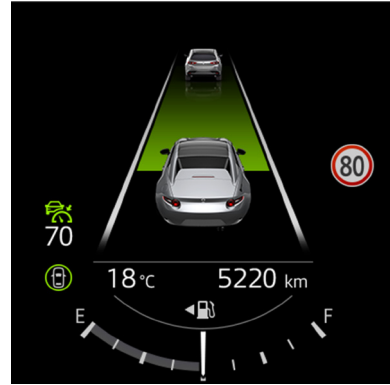
Fig. 6 Meter Display Example of MRCC
