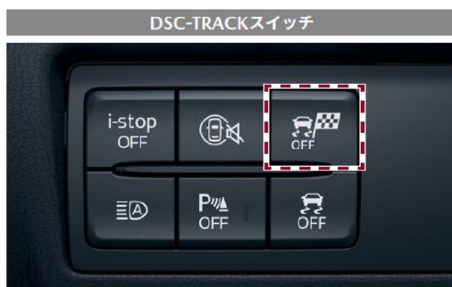
Fig. 11 Human Machine Interface (HMI): Switch of DSC-Track
