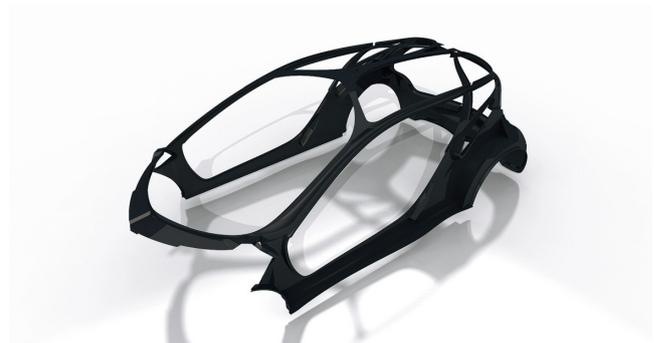
Fig.7 Upper Body Structure of KIYORA
