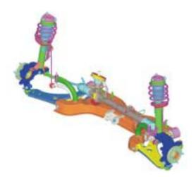
Fig.1 Front Suspension & Steering
