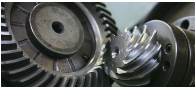
Smoothly meshing hypoid gears allow cars to run with less noise and better stability
